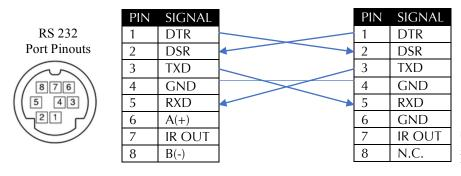
Note: This cable is 4 pieces: 1-A 'straight' RJ45 to DIN cable 2-A 'null-modem like wired' RJ45 to DIN cable 3-Two RJ45 to RJ45 connectors.
